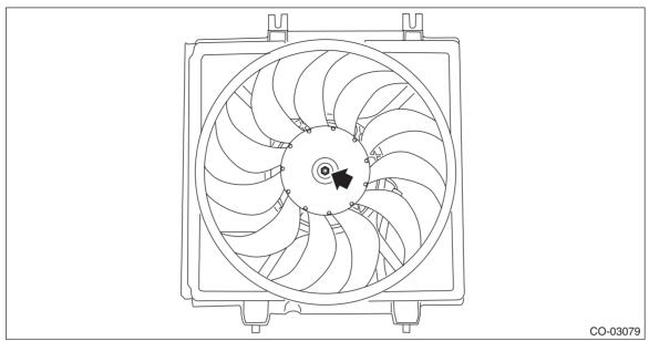
3) Disconnect the sub fan motor from the radiator sub fan shroud.
