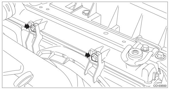
6) Remove the radiator sub fan and fan motor from vehicle.
